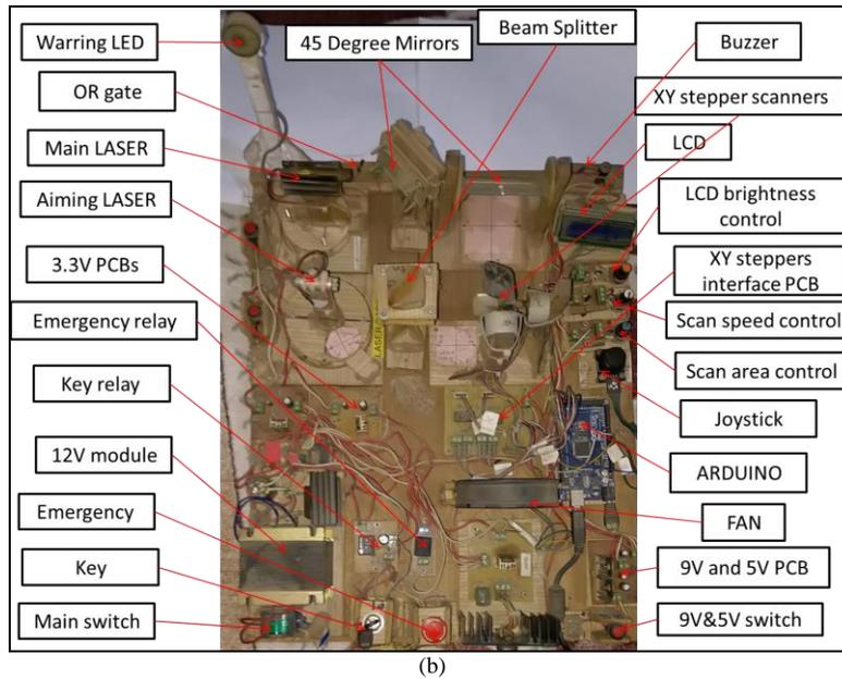
Fig. 1. (a) Block diagram, (b) Real photograph of the proposed optical prototype
