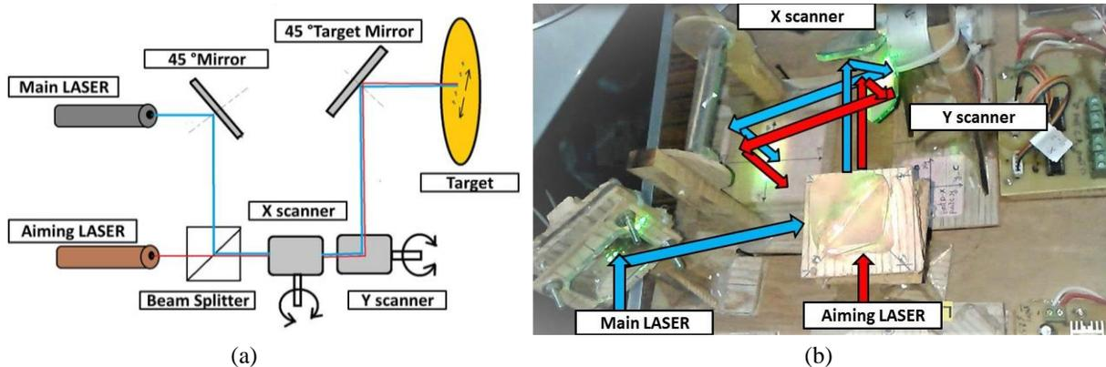
Fig. 2. (a) Schematic diagram of the optical pathway, (b) Real photograph of the optical configuration
