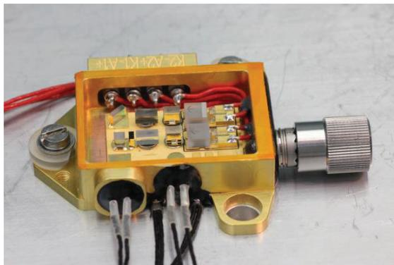
Figure 2: Unsealed unit of Raman Laser Module from Flight Model batch.
