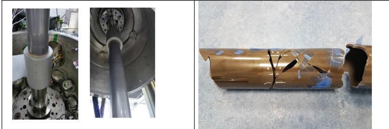
Figure 6. tensile testing of scale 1 tube : test facility (left); tube parts after failure (fractography analysis)(right)
