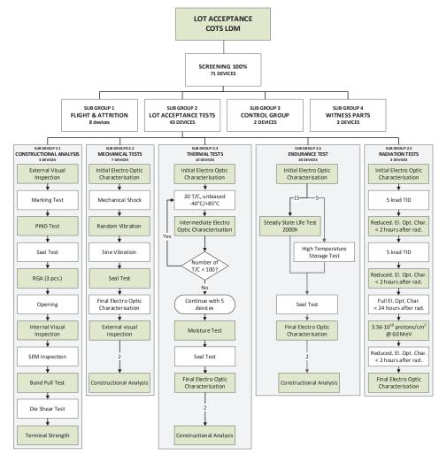
Figure 2-1 LDM LAT Test flow.
