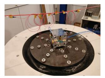
Figure 2-5 Vibration test setup
