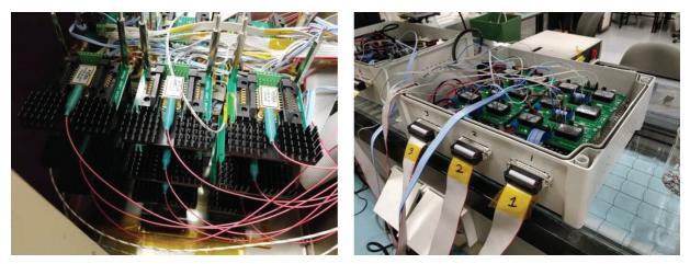
Figure 2-7 Endurance test setup. Left: Lasers mounted in sockets . Right: Thermo-electric controllers.
