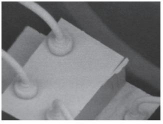
Figure 2-8 SEM picture of laser chip, showing small piece of top metallization remaining after die cutting.
