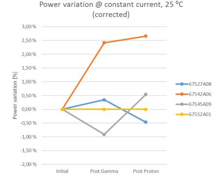
Figure 2-10 The drift in optical power due to radiation environment. The measurements were corrected to account for variation in the test setup. Reference LDM 67552A01, which was not radiation tested, was used for the normalization.
