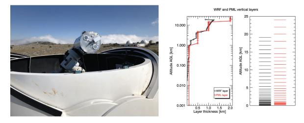
Figure 4. Left: PML instrument installed on the Calern Observatory. Right: Vertical resolution reached by the PML (red) and by the forecasting tool (black) (see section 2.3)
