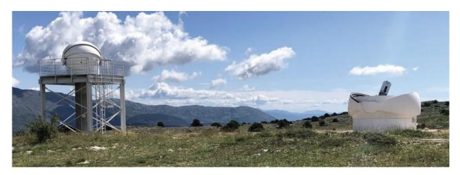
Figure 1. CATS station installed on the Calern Observatory. The left instrument is the G-DIMM, and the right one is the PML.
