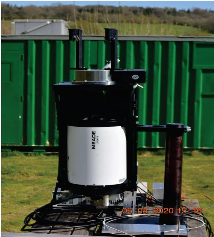
Figure 4. The figure shows the MEADE telescope, two 45 degree mirrors that turns the bistatic into a monostatic optical lidar configuration, the elliptical scanning mirror. Not present in this configuration is the bandpass & Rayleigh filter.
