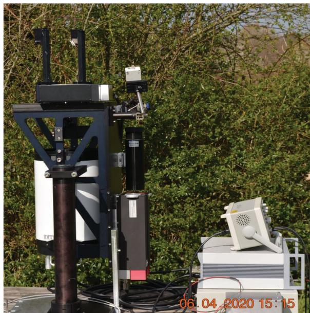
Figure 3. The CWL used in the experiments. It can be seen, on the left, the small transmitter attached to the lidar frame together with the receiver telescope. To the right, it is visible part of the receiver electronics. The laser transmitter is a commercial French-built TEEM laser, multi-mode, un-stabilized, providing o/p energy of  $\sim 20\mu\text{J}$  @ 1 KHz @ 355 nm. On top of the laser it can be seen beam expander with a Newport Scanner & mirror mount.
