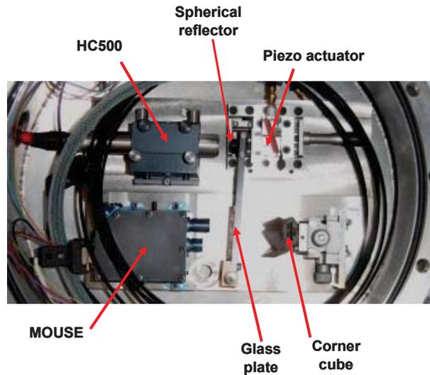
Fig. 4: photograph of the test bench
