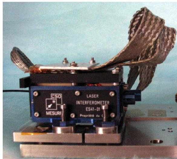
Fig. 9 : MOUSE with thermal braid
