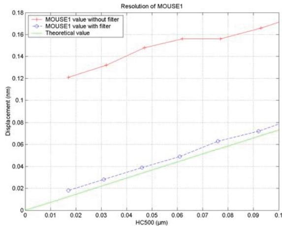
Fig. 6 : Results on resolution tests (part of the figure above)
