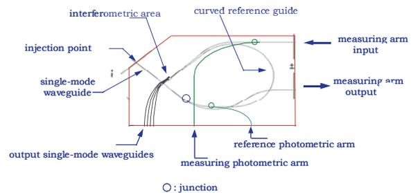
Fig. 1 : Layout of the optical circuit
