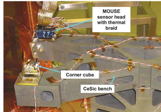
Fig. 12 : Sensor installation on the HSOB
