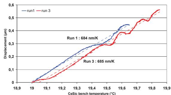
Fig. 13 : Repeatability of CeSiC expansion measurements
