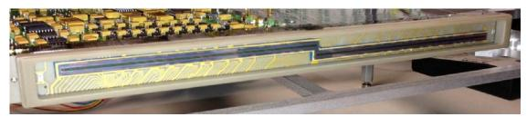
Fig. 4. Front view of BAE Systems CCD21122 mounted on Test Frame
