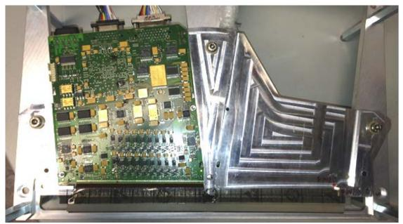
Fig. 3. Top view of BTDI Test Frame and the CCD Controller PCB for one die
