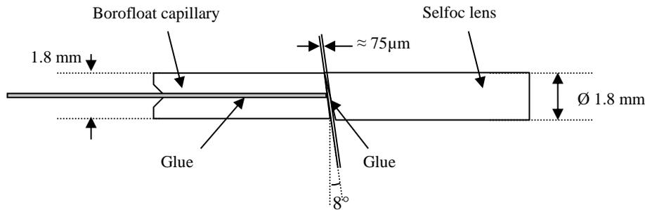
**Fig. 3 :** Collimator design
