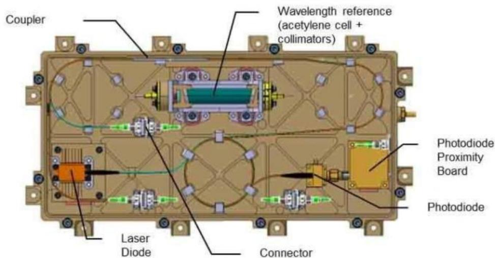
Fig. 5 : Fiber Optical Bench of the MTG Laser
