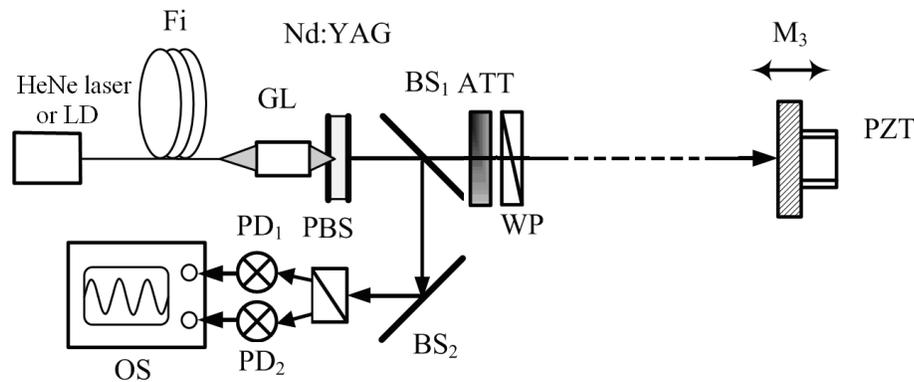
Fig.3 Schematic diagram of microchip Nd:YAG laser feedback with birefringence external cavity. Fi: optical fiber, GL: GRIN lens, ATT: attenuator, WP: wave plate, M3: feedback mirror, BS1,2: beam splitter, PBS: polarized beam splitter
