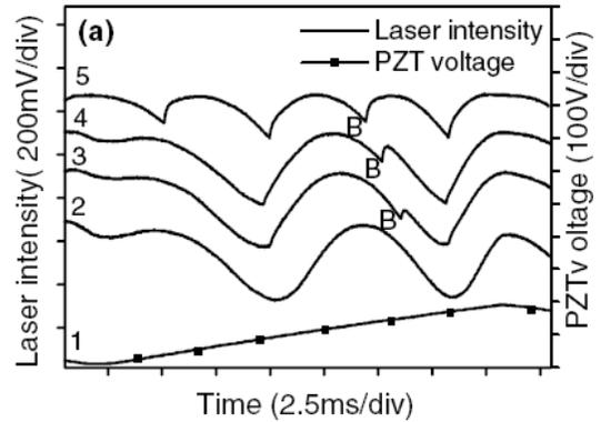
Fig.6 Laser polarization flipping for different phase retardations of birefringence in external cavity
