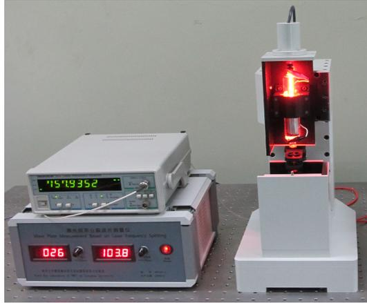
Fig.4 Frequency-splitting wave plate measurement system
