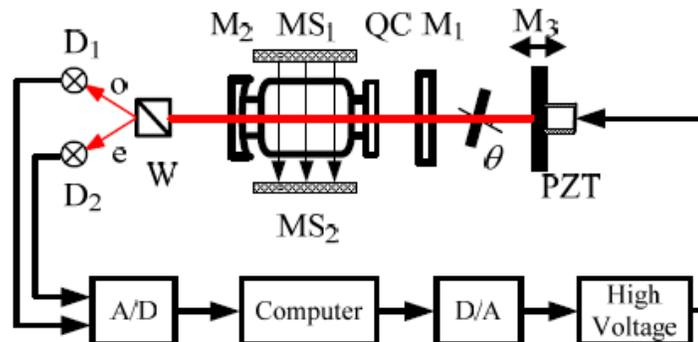
Fig.2 M1, M2: mirrors; MS1, MS2: magnet strips; QC: quartz crystal; M3: external feedback mirror with high reflectivity; PZT: piezoelectric transducer; W: Wollaston prism; D1, D2: detectors
