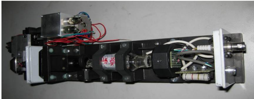
Fig.1 Laser nanometer ruler prototype
