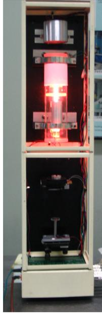
Fig.5 Laser feedback wave plate measurement system
