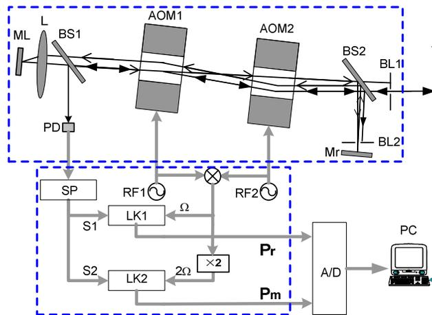
Fig.7. quasi-common-path microchip laser feedback interferometer
