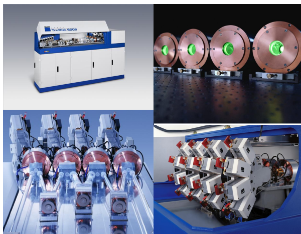
Figure 15: Commercially available 8 kW thin disk laser. Upper left: The entire laser system including chiller, beam switch and controls enclosed in a compact enclosure. Upper right: the four disks inside the pump cavities – the photoluminescence of the disks is visible. Lower left: The resonator setup with four thin disk modules in series, enabling a guaranteed output power of 8 kW at a beam quality of 8 \text{ mm} \cdot \text{mrad} . Lower right: Each pump cavity is pumped with 4 individual stacks of high power diode laser arrays that can be exchanged by a trained operator within a few minutes.
