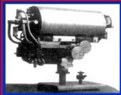
One of first Soviet ruby lasers used for Moon ranging experiments (September 1963) GOI (Leningrad), Design Bureau № 16
