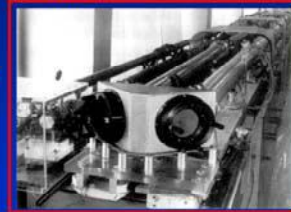
High power carbon dioxide laser - 1 Kw, July 1966 Research Institute № 801
