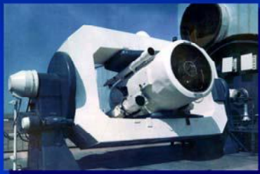
TG-1 1,3 m laser telescope and beam director
