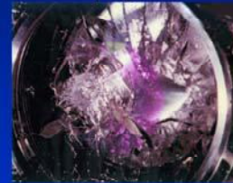
400 mm Raman laser glass optics damaged by laser radiation . Fused quartz was used later
