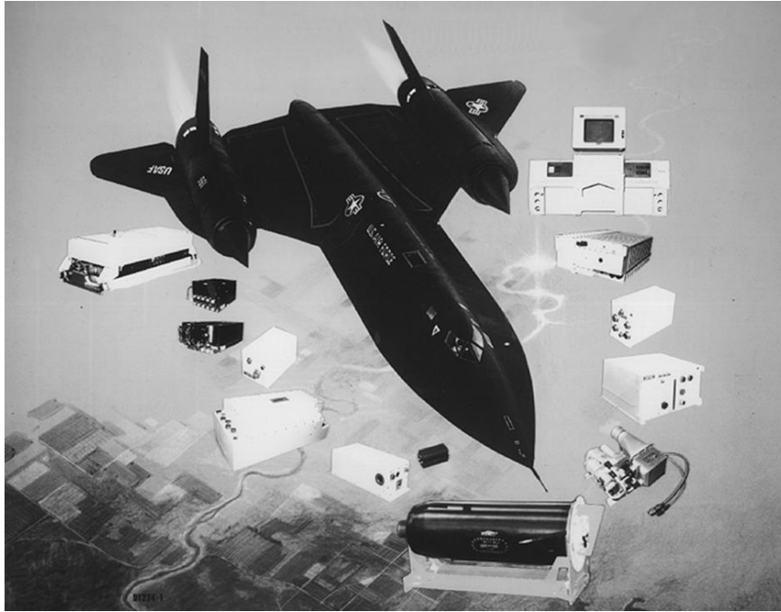
Figure 15 – A picture of SR-71 and ASARS-1 Equipment.
