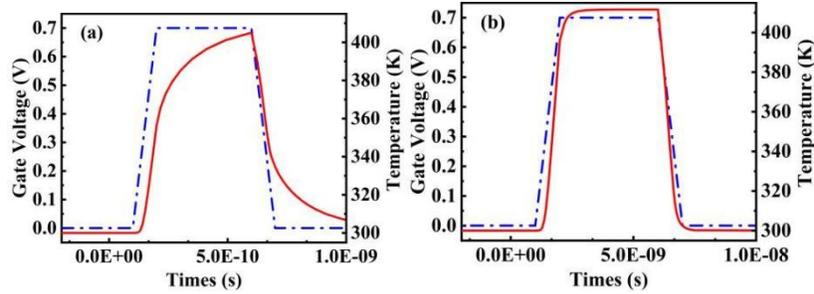
Figure 8. Transient response curves (a)  $F = 1\text{GHz}$  and (b)  $F = 100\text{MHz}$ .
