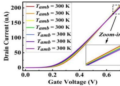
Figure. 9 Impact of ambient temperature on the transfer characteristic.
