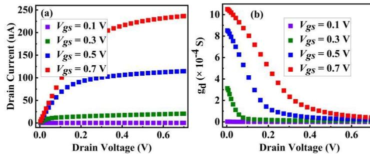
Figure 4. N-type NS-GAAFET (a) output characteristics and (b) conductance characteristics.
