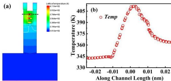
Figure 7. N-type NS-GAAFET (a) lattice temperature distribution and (b) lattice temperature distribution curve along the channel length.
