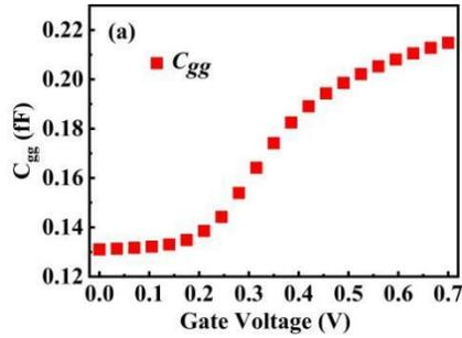
Figure 5. Gate-to-gate capacitance versus gate voltage.
