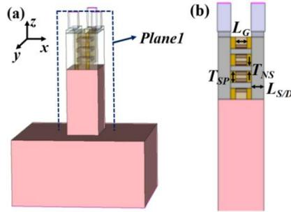
Figure 1. N-type NS-GAAFET (a) the 3D structure and (b) the 2D cross-section along plane1.
