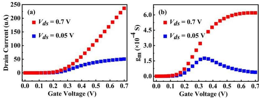
Figure 3. N-type NS-GAAFET (a) transfer characteristics and (b) trans-conductance characteristics.
