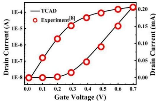
Figure 2. The transfer characteristic curves of the calibrated device and the experimental data.
