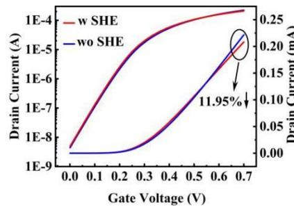
Figure 6. The influence of SHEs on the transfer characteristic.
