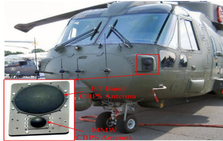
Figure 2. Convectional antenna design with discrete apertures.
