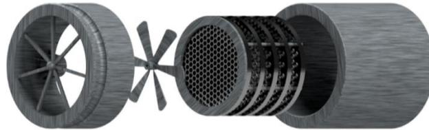
Figure 18. Structure diagram of flue gas treatment part
