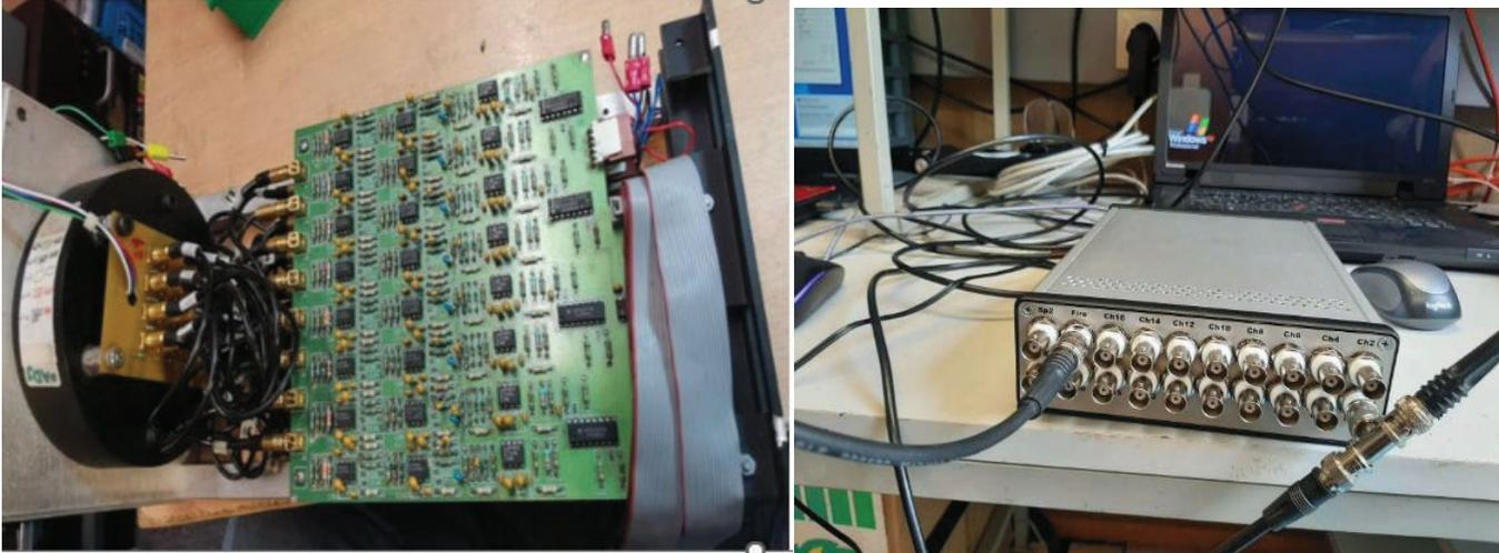
Figure 11. The figure on the left shows a Photek 24-Channel array PMT-MCP array detector and its electronics
