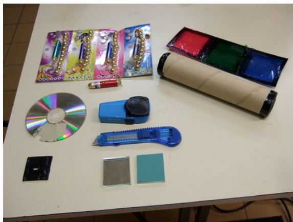
Figure 12. Low-cost equipment used in ALOP: inexpensive lasers, diffraction gratings from discarded CDs, slits scratched into coated mirrors, cellophane color filters and spectrometer made from a diffraction slide.
