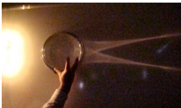
Figure 13. Low-cost cylindrical lens—clear plastic food container filled with water.
