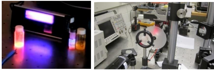
Figure 2. Photos of two experiments of the OPT 204 lab class. LEFT (from a Zoom video recorded in 2021 for remote students): Calculation of sizes of colloidal nanocrystal quantum dots from spectral measurements using Schrödinger equation. RIGHT: Photon statistics measurements from a pseudothermal source.
