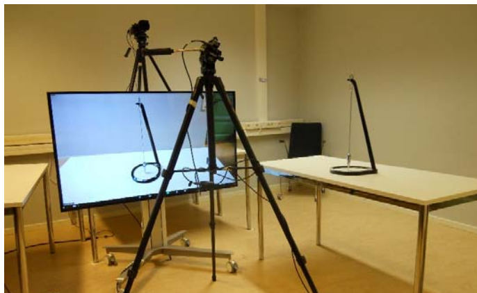
Fig. 2. The webcam in the front films a small conical pendulum; the image can be seen on the TV screen. Using the camera on the tripod, optics experiments can be shown and discussed live with students in a virtual classroom.
