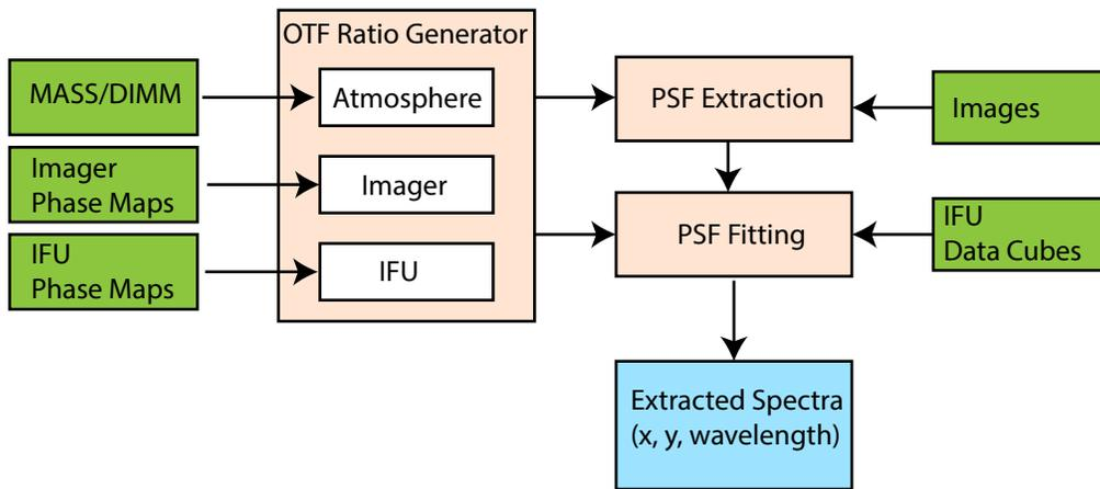
Figure 3. Diagram of the major components of AIROPA-IFU. Green are input data, orange are the AIROPA-IFU software components, and blue indicates the output.
