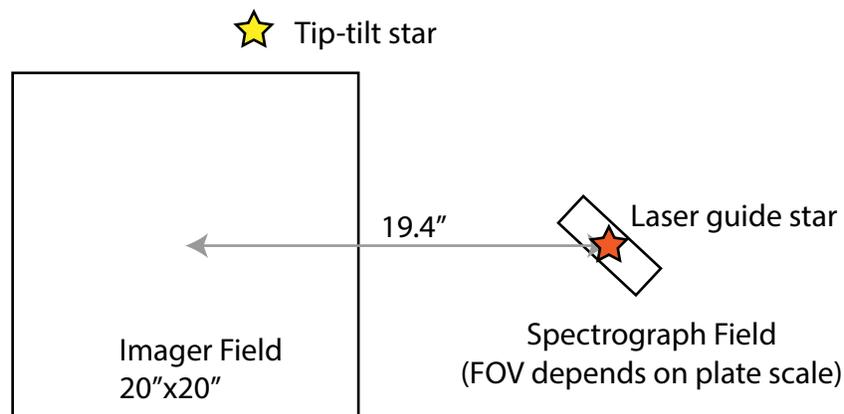
Figure 2. The instrument layout for the OSIRIS IFU. OSIRIS consists of two instruments, an imager and an IFU. The two instruments are about 20" apart in the focal plane. Typically, observations with the IFU will have the laser guide star centered on the spectrograph. A major advantage of OSIRIS is that both instruments can be used simultaneously, which enables observations of PSF references on the imager.
