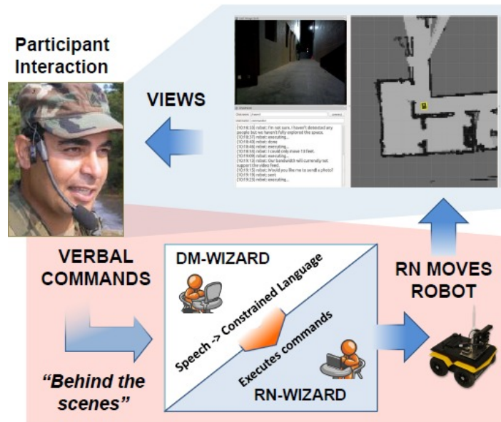
Fig. 7. The participant provides instructions, unaware that the robot is composed of two wizards. The Dialog Manager (DM) wizard translates spoken language commands into a constrained action list for the Robotic Navigator (RN) wizard to execute. Map updates, image data, and the robot's dialogue responses are sent to the participant through a multimodal interface (upper right) [37,38].
