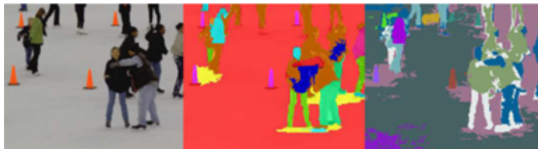
Figure 4. Comparison of segmentation output for our technique which directly models semantics without regard to locality, and hierarchical graph-based (GBH) segmentation which emphasizes segmentation coherency using strict locality rules. USSL, ARL’s approach labels all four traffic cones consistently (column two), whereas GBH assigns unique labels to each cone (column three) [32].
