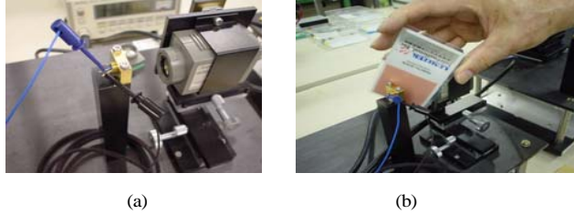
Fig. 6. (a) the laser diode attached to the plate and a power meter, (b) an infrared sensor plate for detecting the light from the laser diode.
