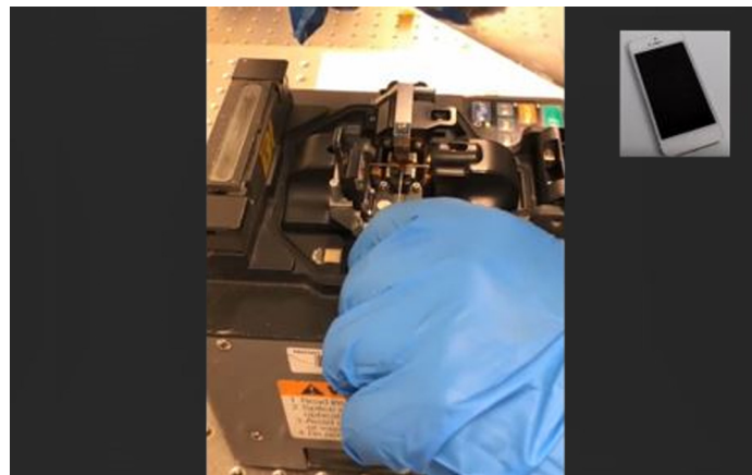
Fig. 17 (From a recorded Zoom video by an iPhone camera.) Fusion splicing of the optical fibers during a remote lab. A Marshall camera positioned on a cart in a small room did not permit recording of this delicate procedure in detail.
