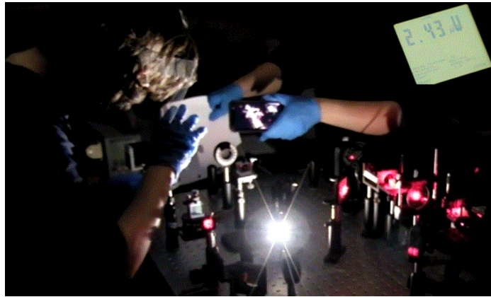
Fig. 12 (From a recorded Zoom video by a Marshall video camera). A single-photon interference lab experiment recorded in the darkness. An inset shows the power meter readings immediately after the lights were turned off.
