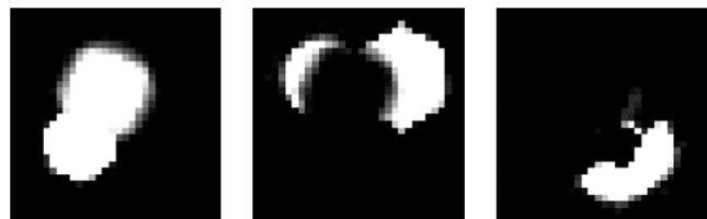
Fig. 11 Experimental demonstration of 3-D AFSI for 32 \times 32 scenes. The reconstructed scenes for the near, mid-, and far ranges (from left to right) with full AFSI adaptation. Images shown are with 48 projections, for a compression factor of 21. The measured amplitudes of the objects are 1.6, 1.2, and 1.3.
