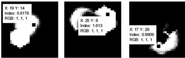
Fig. 8 Estimation of scenes and scene reflectivities for scene reflectivities of 0.9, 1.6, and 1.1 for the near, medium, and far ranges, respectively. The high-noise regime ( \sigma_n = 0.4 ) was used here to compare with the experimental results, which have similar noise levels. The reflectivity levels measured for the estimated scenes at each range were constant over much of the objects seen in each scene. Ninety-six Hadamards were projected for a compression factor of 11.
