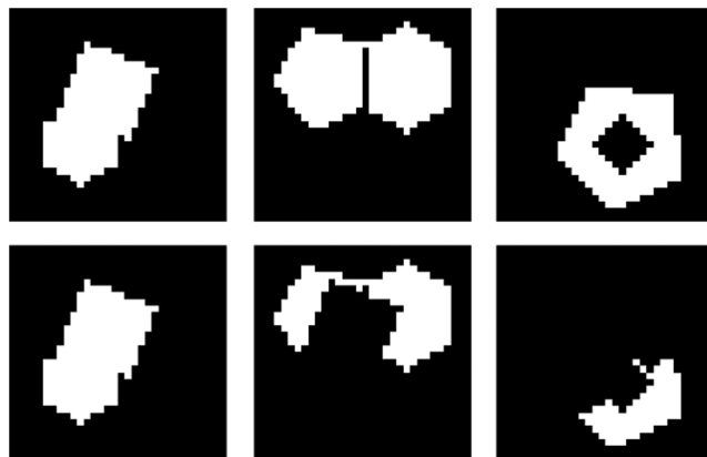
Fig. 1 Top row: 32 \times 32 actual scenes from the closest range on left to farthest range on right. The white and black areas have reflectivity 1 and 0, respectively. Bottom row: 32 \times 32 obstructed images of the scenes as viewed by three-dimensional (3-D) adaptive feature-specific imaging (AFSI) imager after each scene is obstructed by the front objects.
