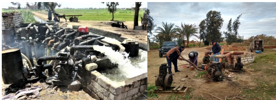
Fig. 4 Examples of small, movable diesel pumps in rural Egypt that are prone to failure and in constant need of repairs. (a) Movable pumps and (b) stationary pumps (source: authors).
