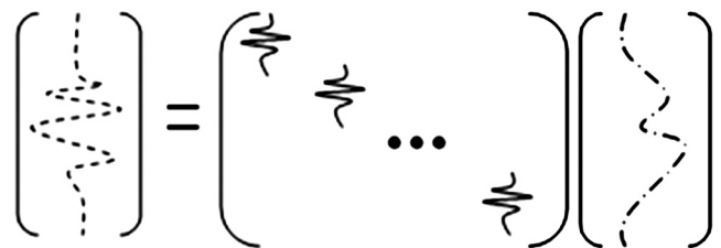
Fig. 3 Visual aid of Eq. (10): dashed line = detected signal I(t) ; solid line = phase-shifted pulses O(t - j\Delta t) ; dash-dot line = profile P(z) .
