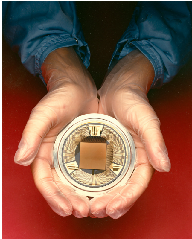
Fig. 15 STIS (1024 \times 1024)-pixel coincidence-anode array (courtesy Ball Aerospace).
