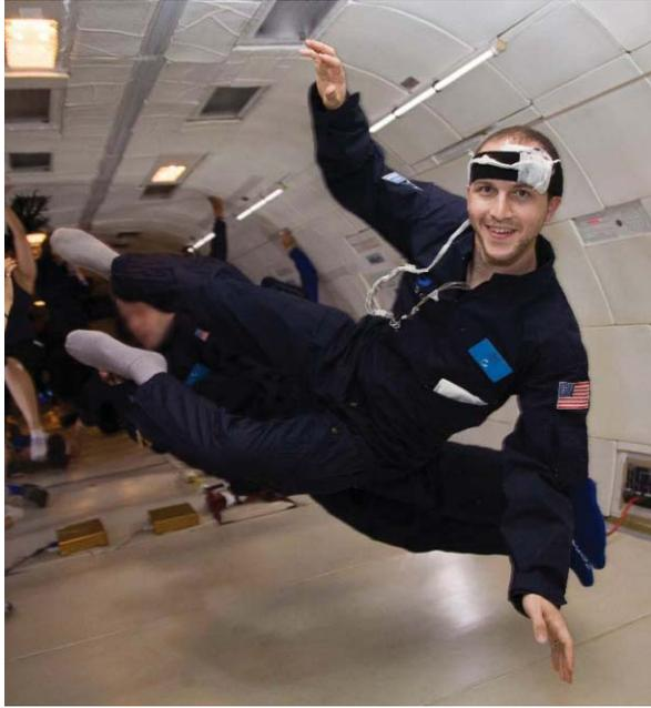
**Fig. 6** *In vivo* hemodynamic monitoring using aNIRS during parabolic flight. Wearing NINscan, the subject went through six parabolas simulating the gravity on Mars, six parabolas simulating Lunar gravity, and four parabolas simulating spaceflight. The systemic and cerebral hemodynamics were monitored continuously during the flight, together with simultaneous re-registered acceleration, respiration and ECG. [The authors have written permission to show the participant's face.]
