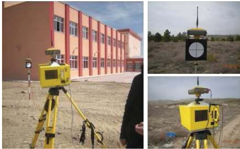
Fig. 1 Laser scanning with sensor integration of terrestrial laser scanner (TLS) and global navigation satellite system (GNSS).
