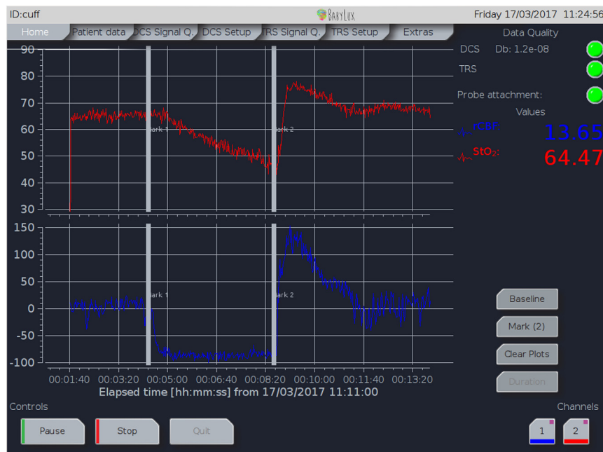
Fig. 2 Screenshot of the home window of the device during a cuff occlusion of an adult arm. Time series of the oxygen saturation (top) and relative BFI (bottom) are reported in the time plot. Color dots on the right top corner represent the optical quality of the data collected and the attachment of the probe as monitored by a capacitive sensor placed on the probe.
