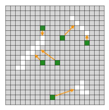
**Fig. 3** Schematic of a frame containing particle tracks (white pixels) and valid events (green pixels). The image segmentation would identify three particle tracks in this frame. Orange arrows indicate the distance between each valid event, defined by the maximum pixel of the  $3 \times 3$  island, and the nearest particle track or MIP pixel.
