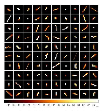
**Fig. 2** Images of a small sample of individual particle tracks, with the color scale in keV. Pixels shown are equivalent to 130  $\mu$ m WFI LDA pixels, so the image sizes are not the same and scale with the size of the tracks.
