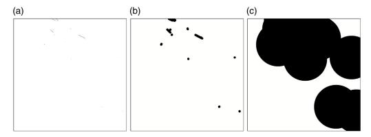
**Fig. 8** Example of calculating the fractional remaining area after SAC masking. (a) A single, full LDA frame with several particle tracks; (b) masking with a radius of 10 pixels around each particle track pixel; and (c) masking with radius 200 pixels. Overlapping masking circles require us to empirically determine the remaining area.
