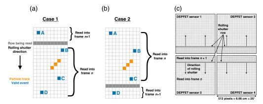
**Fig. 13** Schematic showing the effects of the WFI LDA rolling shutter on SAC from the point of view of a MIP track that accompanies four valid events. (a), (b) The two major cases, where the MIP track is below (case 1) or above (case 2) the current readout row, which moves downward in these depictions. (c) A depiction of the full LDA focal plane. We assume the rolling shutters are synchronized between the four DEPFET sensors and move in the directions shown.
