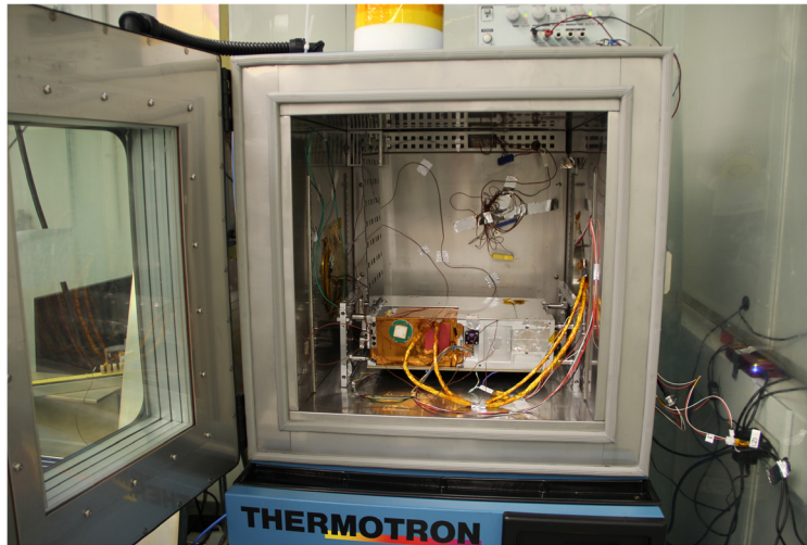
Fig. 9 DeMi spacecraft installed in thermal chamber. Photo credit: MIT Lincoln Laboratory.
