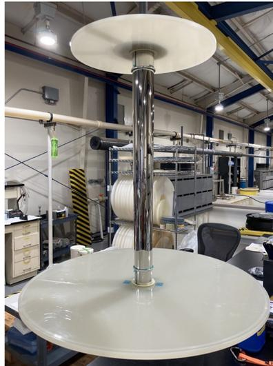
**Fig. 12** Seventy-centimeter-long mandrel with differential shield diameters and copper strip gaskets (picture credit: NASA).
