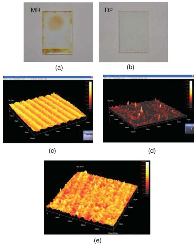
**Fig. 3** (a) Adsorption conditions of MR dyes on the substrate. (b) Adsorption conditions of D2 dyes on the substrate. (c) Surface relief structures of the adsorbed MR dyes observed from an atomic force microscope. (d) AFM observation on substrate in D2-doped sample. (e) AFM observation on substrate after the erasing process in the MR-doped sample.
