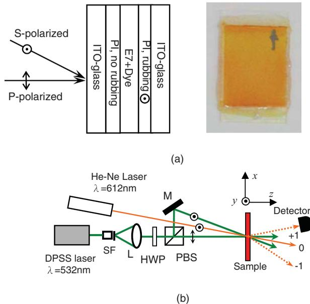
**Fig. 1** (a) Sample structure of a dye-doped liquid crystal film. (b) Schematic diagram of the experimental setup. SF; spatial filter, L; lens, HWP; half-wave plate, PBS; polarized beam splitters, M; mirrors.
