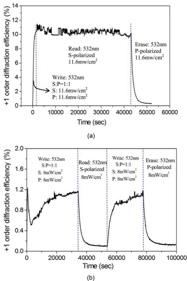
**Fig. 2** (a) Evolution of +1 order diffraction efficiency during a write-read-erase process for a MR-doped liquid crystal film. (b) Evolution of +1 order diffraction efficiency during a write-read-write-erase process for a D2-doped liquid crystal film.
