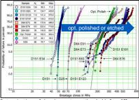
Determination of breakage stress threshold for different surface conditions by fitting the 3-parameter Weibull statistics
