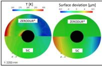
Relative response of ZERODUR® and SiC primary mirrors: (left) temperature smoother for SiC; (right) ZERODUR® shows smoother surface deviation. high diffusivity fails to compensate for low CTE in terms of surface deviation [2].
