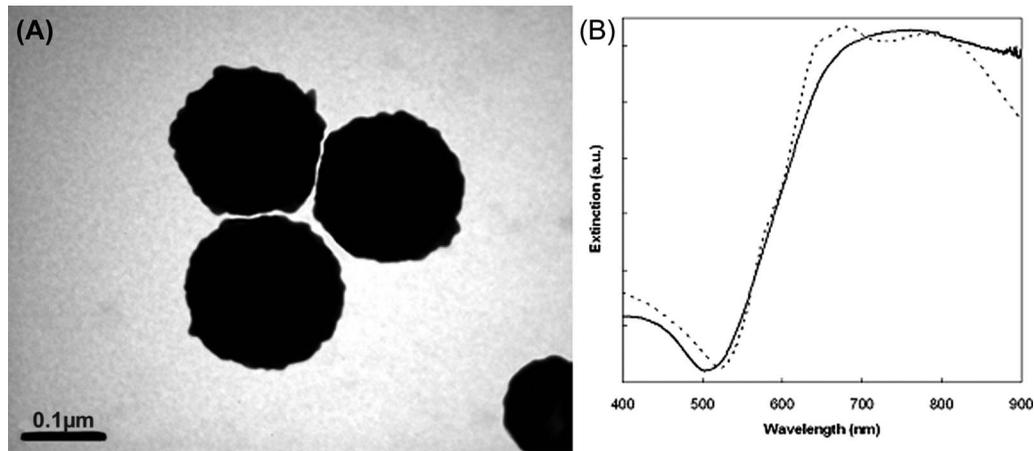
**Fig. 2** (a) Electron micrograph of gold nanoshells with an 81-nm radius dielectric silica nanoparticle core and 23-nm-thick gold shell. (b) Measured UV-VIS extinction spectrum of the synthesized gold nanoshells (solid line). The theoretically calculated extinction spectrum of gold nanoshells of the same dimension as derived from the Mie theory is shown for comparison (dotted line).
