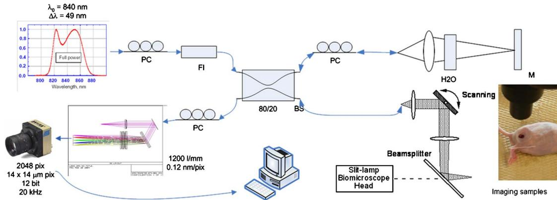
**Fig. 1** The schematic of the spectral domain OCT imaging system used in this study. Image courtesy of Bioptigen Incorporated. The setup for imaging various samples such as phantom and small animal models is shown as an inset in the figure.
