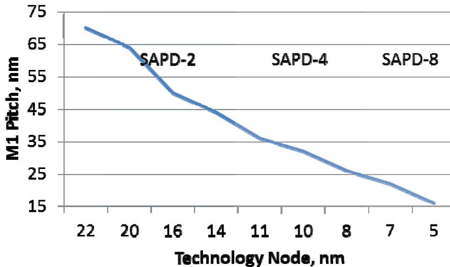
Figure 2. Metal-1 pitch for sub-22nm logic technology nodes.
