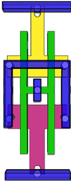
Figure 1a. 2D style layout of logic inverter.
