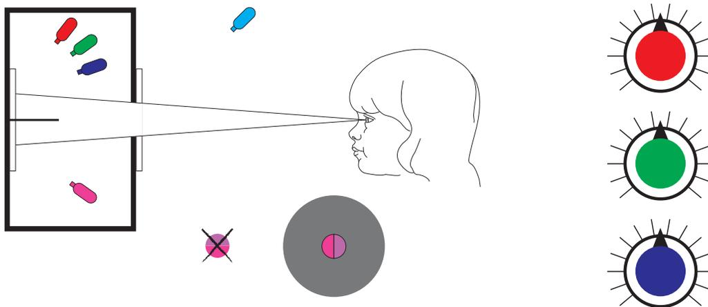
Figure 7. Elements and steps of the color matching experiments. The three knobs at right are turned until the two halves of the bipartite field match. If a match cannot be achieved, a primary source is moved to the other side to desaturate the test color; the corresponding knob is given a minus sign. The optional light source outside the box can be used to create a surround for adaptation.
