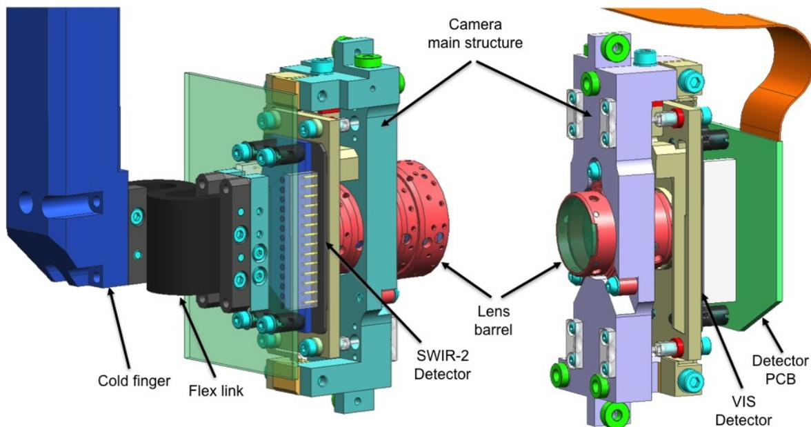
Fig. 5. SWIR-2 and VIS camera assemblies
