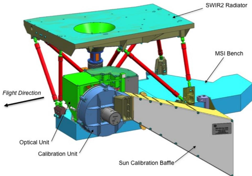
Fig. 2. The VNS instrument
