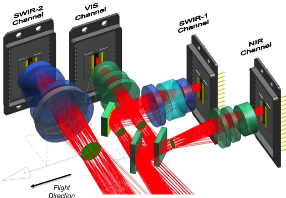
Fig. 3. VNS optical configuration
