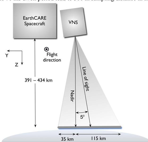
Fig. 1. VNS observing configuration
