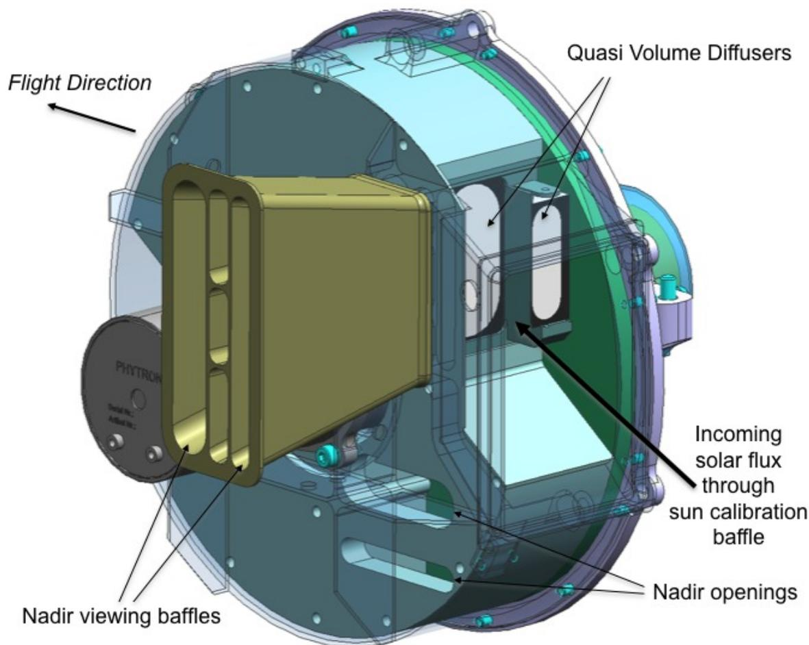
Fig. 4. VNS calibration mechanism
