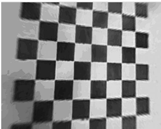
Fig. 9 The result of correction of the fisheye camera distortion after basic calibration.
