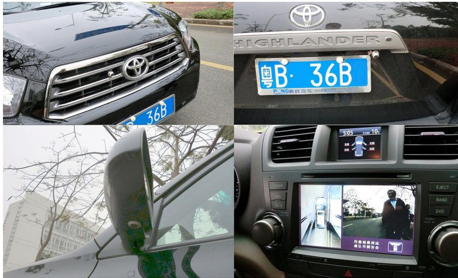
Fig. 5 PPAS installed in a Toyota Highlander.
