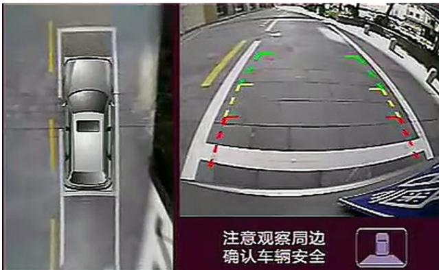
**Fig. 16** Top-view image after mosaicking in final version of PPAS.
