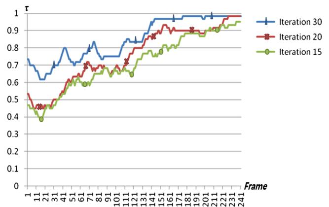
**Fig. 9** Real-time tracking confidence with different numbers of iterations at individual image frame ( $\epsilon = 0.15, \alpha = 0.2, \gamma = 0.95,$  and  $\delta = 20$ ).
